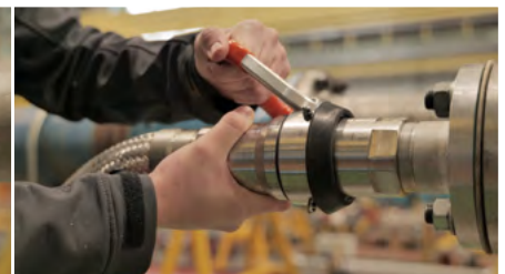
3. TWIST 1/3 TURN CLOCKWISE TO LOCK IN PLACE & RELEASE FLOW
